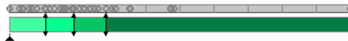
Figure 4. Visual appearance of the compound slider. Three slider pointers (vertical lines with small triangles at both ends) divide the interval into 4 classes. In the dot plot above the slider the grey circles represent values of the attribute.
