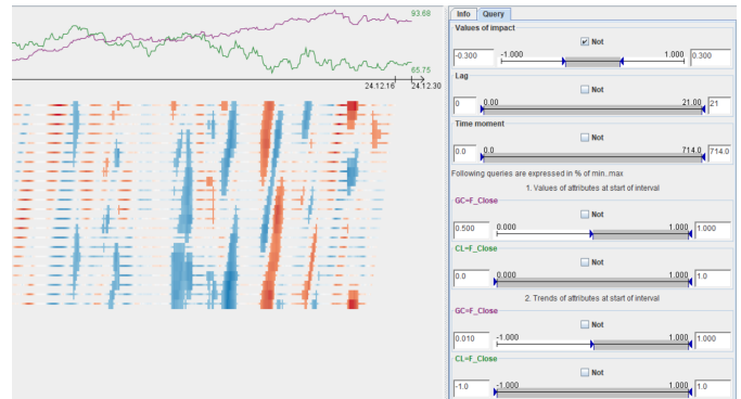
Fig. 7: Ikat plot (Figs. 5,6) after applying a dynamic query [2], as shown on the right. Cells of the \tau matrix that do not meet the query conditions are visually de-emphasized.
