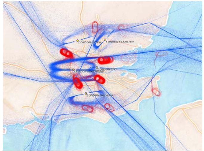
Fig. 8. The final parts of the trajectories of the flights that arrived to London. The holding loops are highlighted in red.
